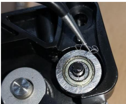
Use supplied tweezers from the 3D printer toolkit to remove debris
