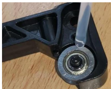
Dab the bearing with the plastic tube to release some Inox
