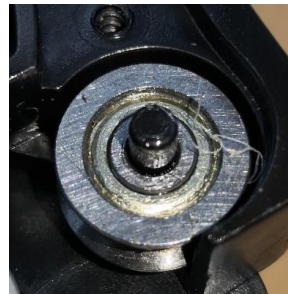
Any plastic filament found on bearing needs to be removed
